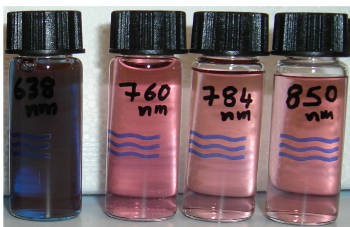
Figure 1: Gold nanorod solutions of 10 ml final volume of batches spanning along the far visible up to near infrared (NIR) region of spectrum. The batches of gold nanorods (from left to right) have longitudinal plasmon peaks of 628 nm, 760 nm, 784 nm and 850 nm respectively.
